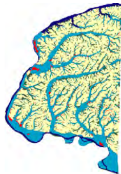
Figure 5. Comparison of simulation model to digitized floodplain. Areas of disagreement are colored red (digitized as floodplain but modeled as upland) and green (digitized as upland, but modeled as floodplain). Dark blue indicates areas within water mask.
